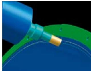
Path corrections allow you to reconcile contour deviations between the CAD model and the real component.
