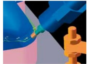
After changes to the spatial orientation of the machine head, the collision check displays only green vectors.
