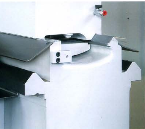
The external prismatic double guides for saddle displacement are protected
