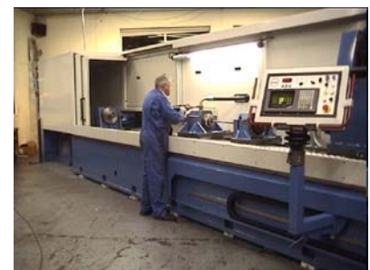
Machine supplied to the aerospace industry to drill hollow ballscrews
