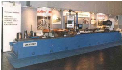
Mollart Boremaster (shown without guards) available with up to 3m drilling depth
