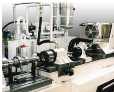
Truck Drive Shaft machine is part of an automatic cell being fed by 5 axis robot
