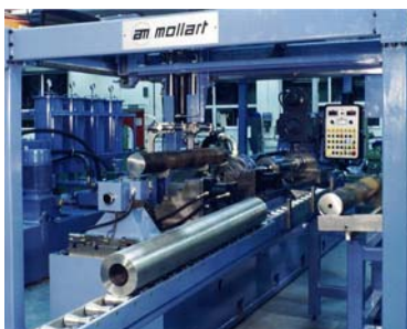
BTA Production Line with gantry loading facility supplied to the oil industry
