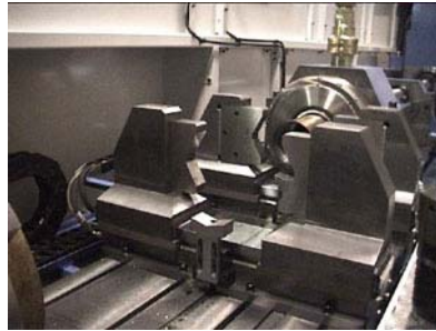
Optional Component Workholding with Hydraulic self centering vices
