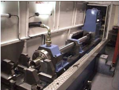
BTA Coolant Pressure Head & Tube Damper tooling to suit all drilling applications
