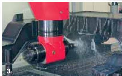
2. Diesel engine manufacturing: machining of diesel engine casings
