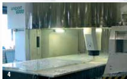
4. High speed routing of large aluminium plates
