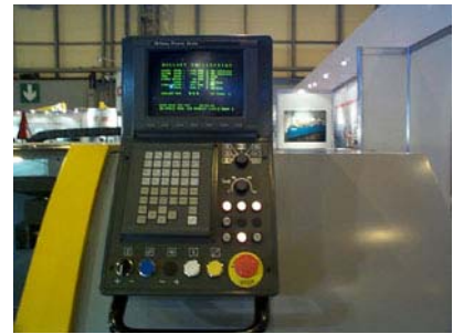
GE Fanuc CNC Control System with programmable spindle feed rate, drilling depth & Process Monitoring
