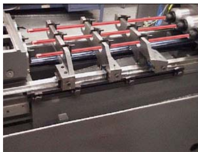
CAM-operated Auto-whipguide positioning
