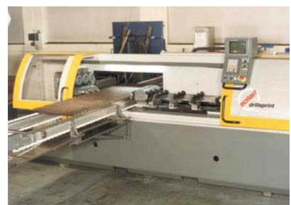
Sporting rifle barrels are fed through the machine with an automatic conveyor that indexes the parts through after drilling. The range of parts were drilling diameters from 5 – 10mm and lengths from 300mm – 750mm and bar max 40mm
