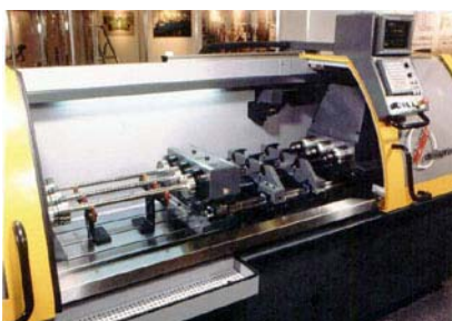
The Drillsprint specialises in gundrilling shafts using counter-rotation units to produce concentric bores where the wall thickness of component is critical, or alternatively tooled with table mounted fixturing for prismatic parts.
