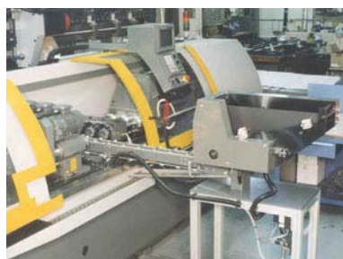
Autoloading of a Windscreen Wiper Shaft. A 3mm x 150mm hole was Gundrilled to allow Washer Fluid to be pumped through into to washer jets mounted on the Windscreen Wiper Blade Arm. The Feeder unit has the capacity to operate for one full shift.
