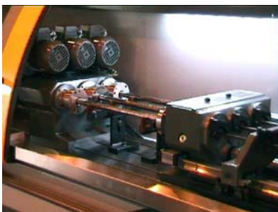
Work rotation Units for maximum concentricity between bore & outer diameter. Parts can also be fixtured on the machine table
