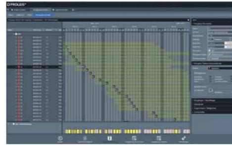
Control center: Display of assignment plan with time frames (above) and machine utilization (below).
