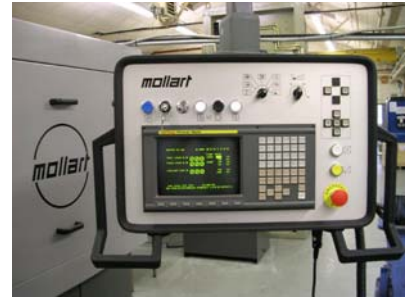
GE Fanuc CNC Control System with Mollart custom programming for simple set up, programmable spindle speeds, feed rate, drilling depth & Process Monitoring
