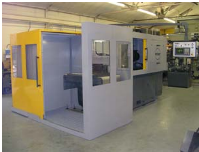
Fully Enclosed Guarding System with other guarding options to suit auto loading options.
