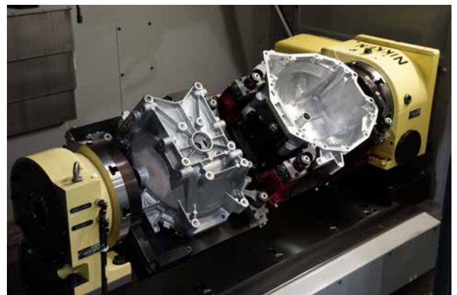
Interface for hydraulic fixtures / rotary / tilt axis for PS Serie
